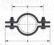
Material/Finish: Carbon steel ☐ 304 stainless steel ☐ 316 stainless steel Plain 🔲 electro-galvanized Designed for supporting and stabilizing vertical pipe runs. Overall length of clamp is shorter than standard to Service:
